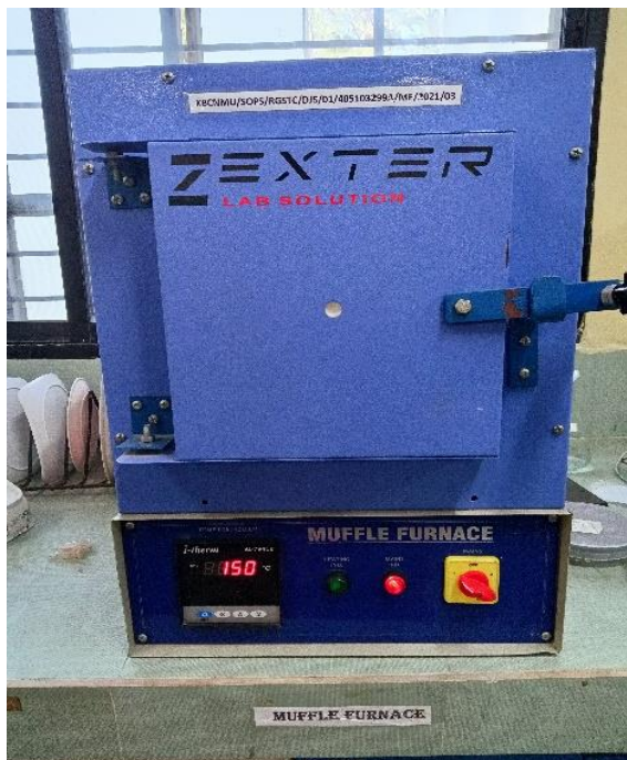
Fig:- The resulting crystal or substance is calcined at 150 °C during 2 h
